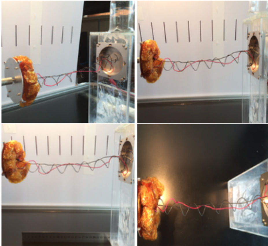
Figure 6.36 Images of the ADDUCT device once the Nitinol helical boom has been deployed.
