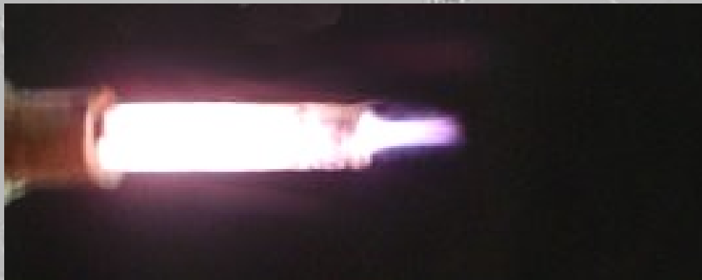
Argon-plasma jet in atmospheric pressure, experimentally observed in Faculty of Physics
