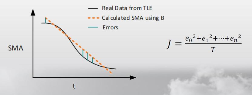
Dividing the cost function by T makes cost function and fitting performances comparable between satellites that have different data and time span.
