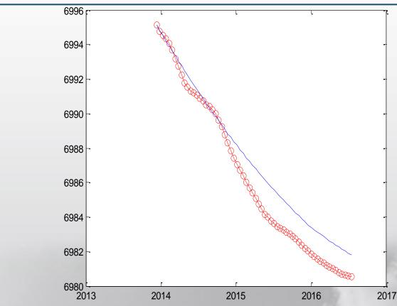
The best case occured for iCUBE-1 satellite and the semi-major axis difference at the end of 2.5 years analysis is smaller than 1 kilometers.
