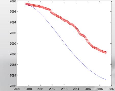
The worst case occured for UWE-2 satellite and the semi-major axis difference at the end of 7 years analysis is smaller than 6 kilometers.
