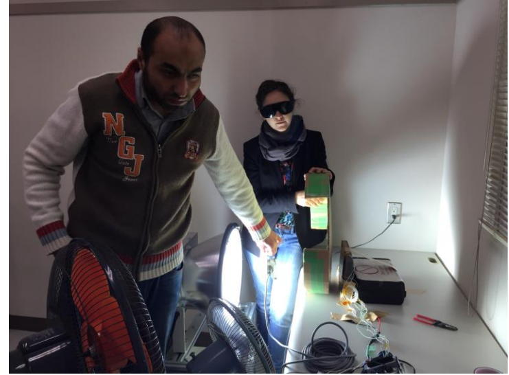
Solar simulator 30cmx30cm area with 1400W/m 2
