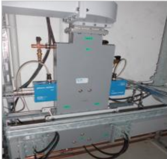
Fig. 1.1 design and manufacturing of the power divider (high energy) and RF phase shifter
