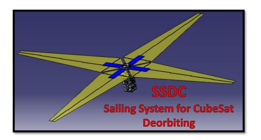
The designed SSDC (Sailing System for CubeSat Deorbiting) allows the deorbiting of a CubeSat by exploiting the free and unused volume offered by the standard solar panels without changing the nominal configuration of main subsystems
