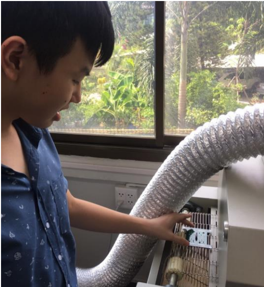
PCB Board is baking in the oven
