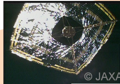
IKAROS (2007-2010) World's first interplanetary solar sail
