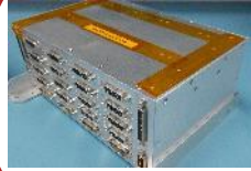
Time Sequencer with Command and TLM interface to LV
