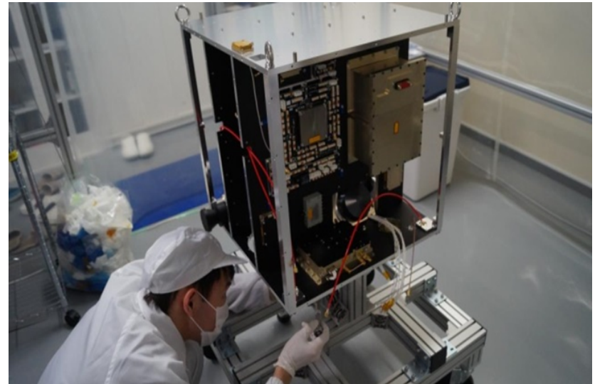
Master and doctoral students of KazNU on internship in Japan: installation and testing of the small satellite UNIFORM 2 (Kyushu Institute of Technology )
